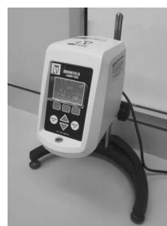
Viscometer used for measuring the viscosity of liquids
