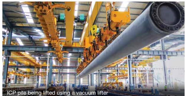
ICP pile being lifted using a vacuum lifter
