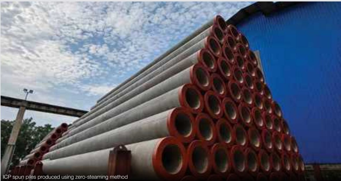
ICP spun piles produced using zero-steaming method
