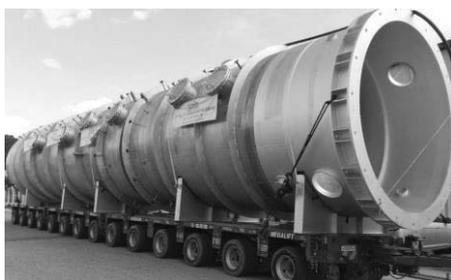
A pressure vessel is a closed container or pressurised tanks that are designed to hold gases or liquids at pressures that are substantially higher or lower than the ambient pressure.
