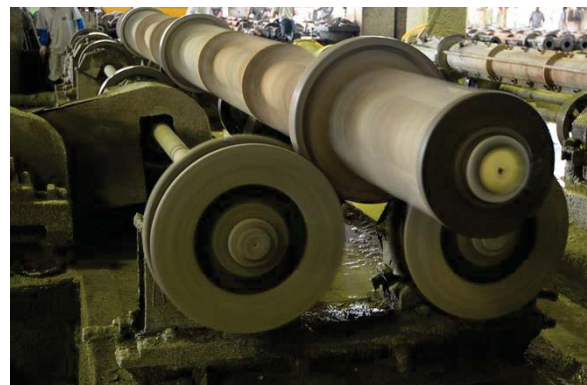
A mould being spun on one of our centrifugal spinning machines
