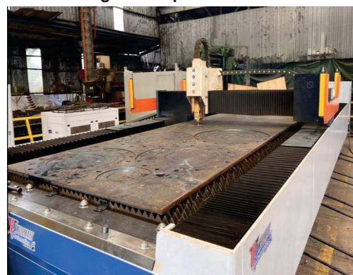
Cutting a steel plate for a mould
