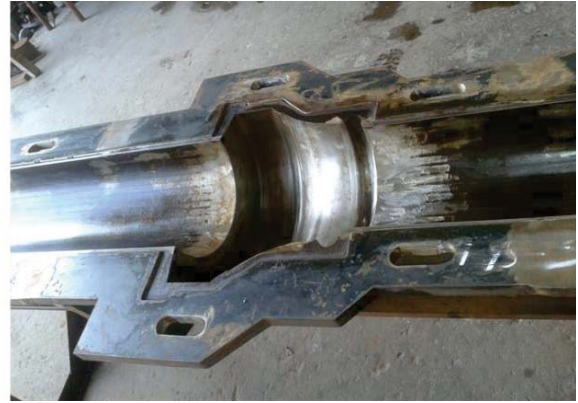
Right: Interior of a mould for decorative poles.
