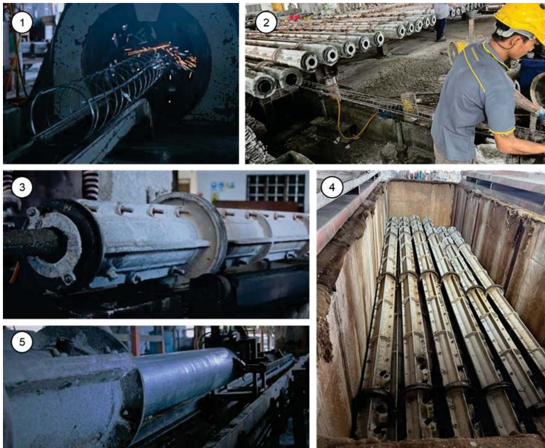
(1) Manufacturing the steel cages (with rods) to serve as reinforcement. (2) Inserting a steel cage into a mould. (3) Injecting concrete into a mould before spinning. (4) Steam curing. (5) Demoulding a spun pole after steam curing.
