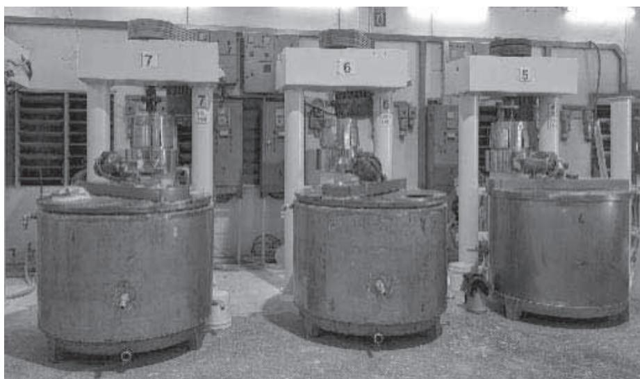
During the wet grinding process, we add several types of chemicals such as dispersing and binding agents into the mixture based on our formulation. These chemicals are added to ensure that the kaolin particles remain dispersed for a certain time in the liquid mixture. Our kaolin dispersions have a shelf life of 4 months before the particles start to settle down and coagulate.
