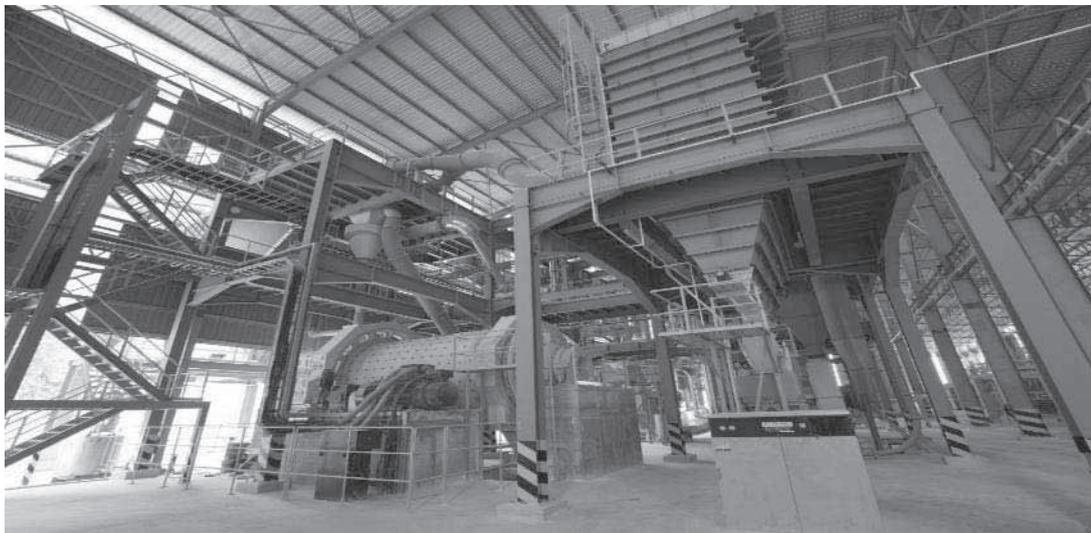
Our GCC production lines are equipped with air classifiers to separate the GCC into different size classes. The air classifier uses an air cyclone and gravitational force within the machine to separate light weight ultrafine particles and heavy coarser particles.
